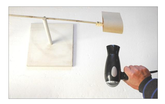
The apparatus is set up with an aerofoil on the right side and a counterweight on the left side. A hair dryer, **see photograph above**, supplies a constant air stream that is aimed straight at the front of the aerofoil. The aerofoil should be placed with the curved surface on the top. As the air flows over the aerofoil, that side of the apparatus will lift up. The air must travel farther over the top of the airfoil, so it travels faster, **see diagram below**. This
