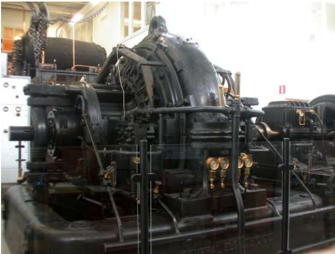
200 kW Alexanderson alternator preserved at the Grimeton radiotelegraphy station, Sweden, the only remaining example of an Alexanderson transmitter.
