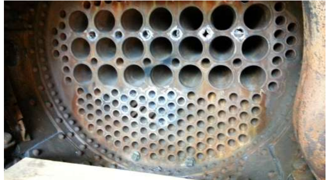
Typical boiler tube plate showing large smoke tubes that can carry the superheater elements and the small tubes which also convey hot gases and help to heat the water. Photo : PR
