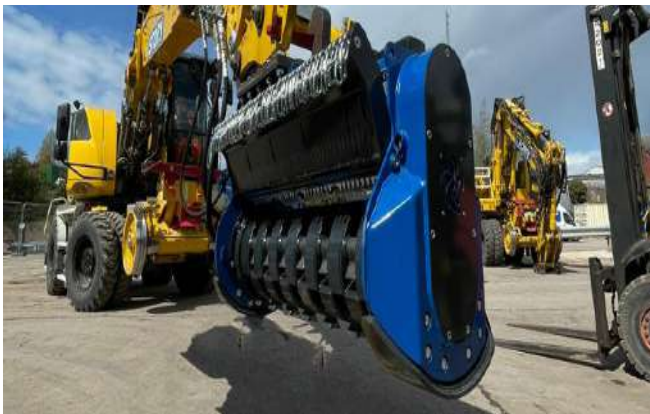
Robustrack LS7 Mulcher Flail to be fitted to LRT's
