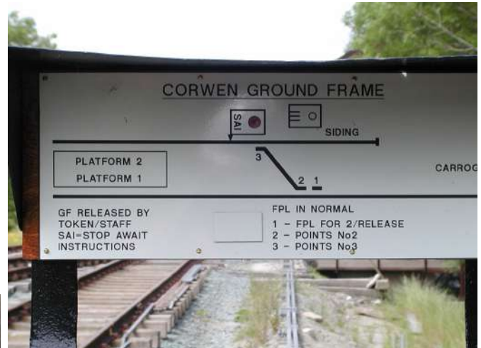
Ground frame diagram for the east end points which allows access to the UP siding and run-round facilities train engines Photo : PR
