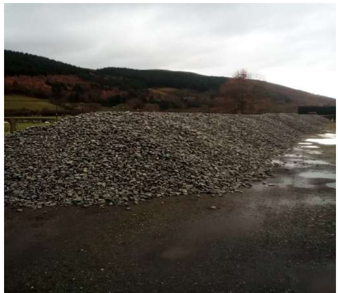
300 tons of Dolerite Ballast in Carrog Yard
