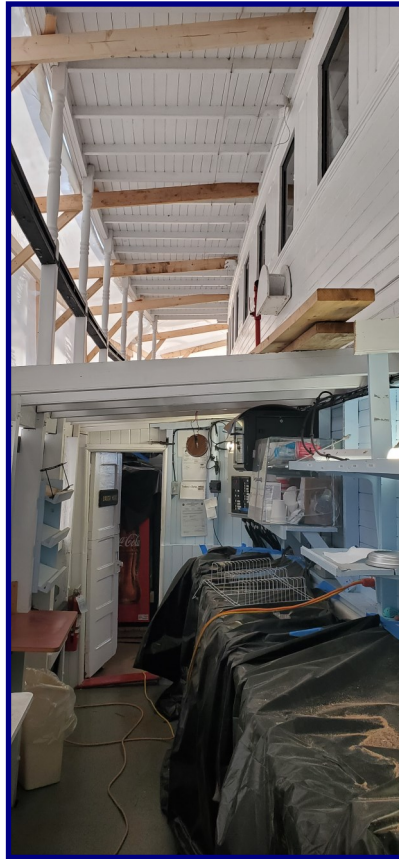
The galley looking aft. Cross beams will be replaced this fall. Planking and fiberglass will be added in the spring.
