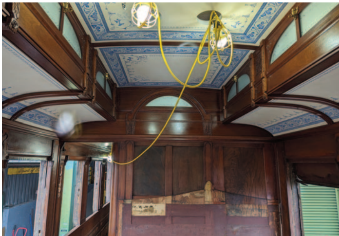
New replica ceiling panel made off of original photos installed in the observation room, replica original ceiling light will top off the room. © J Young
