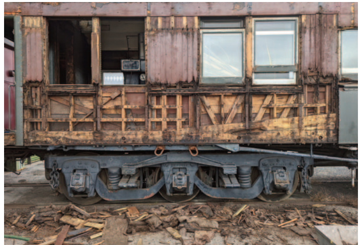
Crews work at removing the rotted siding and horse hair insulation from the A18. © J Young
