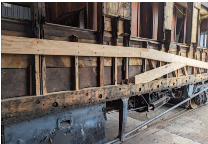
With all the rotted siding removed, structural repairs are being made to make the car solid again. © J Young
