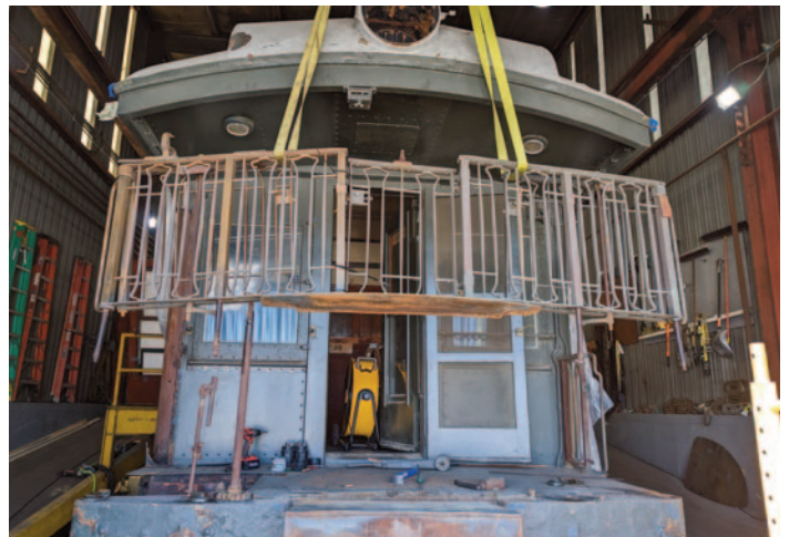
Not original to the car, the observation platform railing was removed to make preparations for a new railing to be made. © J Young
