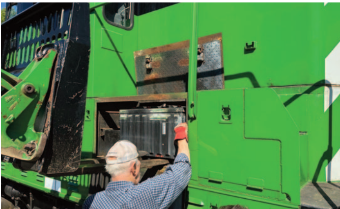
Pete checks clearances between the battery and the compartment on the locomotive.
