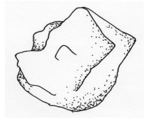
Color: Found in various colors Hardness: 3 Cleavage: Perfect Fracture: Conchoidal Luster: Vitreous/Pearly Streak: White Specific Gravity: 2.711 g/cm<sup>3</sup> Crystal System: Trigonal Uses: Calcite has more uses than almost any other mineral. It is used in construction materials, abrasives, pigments, cement,
