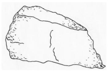
Color: Copper-Red tarnishing to an Iridescent Purplish surface also tarnishing to Black Hardness: 3 Cleavage: Poor/Indistinct Fracture: Conchoidal Luster: Metallic Streak: Gray– Black Specific Gravity: 5.09 g/cm<sup>3</sup> Crystal System: Orthorhombic
