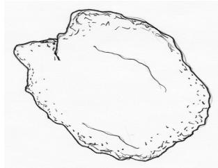
Color: Pink, Rose, Red, Yellowish-Gray, Brown, White, Gray Hardness: 3<sup>1</sup>/<sub>2</sub> Cleavage: Perfect Fracture: Irregular/Uneven Luster: Vitreous, Pearly Streak: White Specific Gravity: 3.7 g/cm<sup>3</sup> Crystal System: Trigonal Uses: Rhodochrosite is an ore of manganese. It may also be carved into
