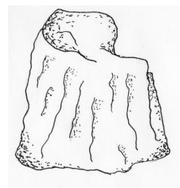
Color: Indigo-Blue or darker. Often iridescent with Purplish, Deep Red, and Brassy-Yellow reflections. Hardness: 1½-2 Cleavage: Perfect Fracture: Irregular/Uneven Luster: Sub-metallic Streak: Shiny Metallic, Lead-Gray to Black Specific Gravity: 4.062 g/cm<sup>3</sup> Crystal System: Hexagonal Uses: It is an important ore of copper. Other Interesting Facts: Covellite is
