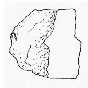
Color: Yellow, Light to Dark Brown, Black, Red Brown, Colorless, Light Blue, Green Hardness: 3½-4 Cleavage: Perfect Fracture: Conchoidal Luster: Adamantine Streak: Pale Yellow to Brown Specific Gravity: 4.096 g/cm<sup>3</sup> Crystal System: Isometric Uses: Primary ore of zinc. Other Interesting Facts: Sphalerite's name is derived from the Greek word sphaleros meaning treacherous.
