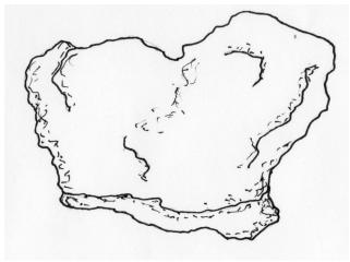
Color: Gray to Grayish Black, turning Bluish when exposed to air Hardness: 2<sup>1</sup>/<sub>2</sub>-3 Cleavage: Poor/Indistinct Fracture: Conchoidal Luster: Sub-Metallic Streak: Grayish Black Specific Gravity: 5.706 g/cm<sup>3</sup> Crystal System: Trigonal Uses: Digenite is an important ore of copper.
