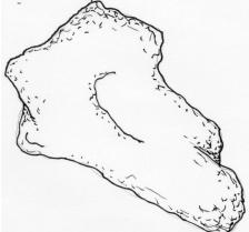
Color: Colorless, White, Gray, Brown, Beige, Orange, Pink, Yellow, Light Red, Green Hardness: 2 Cleavage: Perfect Fracture: Uneven Luster: Vitreous to Pearly Streak: White Specific Gravity: 2.35 g/cm<sup>3</sup> Crystal System: Monoclinic Uses: Gypsum is the primary ingredient in plaster
