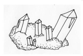
Color: Found in various colors. Hardness: 7 Cleavage: Poor/indistinct Fracture: Conchoidal Luster: Vitreous Streak: White Specific Gravity: 2.66 g/cm<sup>3</sup> Crystal System: Trigonal Uses: Quartz is used in a variety of ways including silica for glass, electri-
